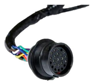
B. Locate the circular male connector C101 on the Under Cab Harness.
