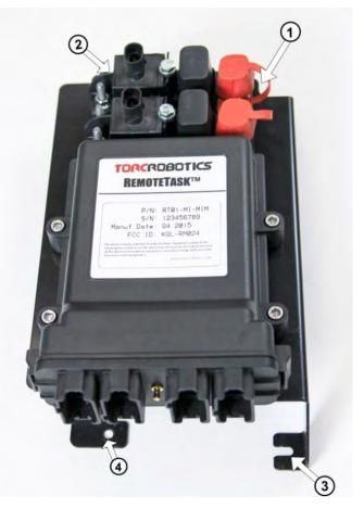
C. Insert the MIM mounting openings onto the loosened screws.
