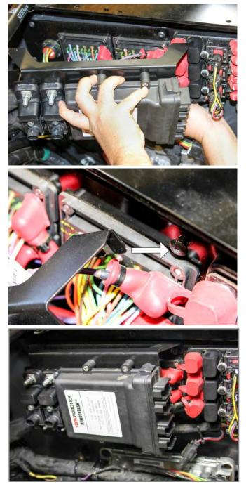
D. Use the T25 TORX driver to tighten all four screws. Ensure that no existing wires are pinched by the MIM.
