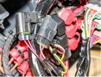
**4. Secure the harness.** Ensure the Machine Interface Harness connectors are routed neatly. Tighten all zip ties to secure the MIH. Clip zip tie ends.
