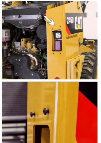
B. Use the T30 TORX driver to loosen the four screws.
