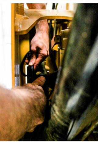
E. Use zip ties to loosely secure the connector cable to the rear electrical lighting harness. Allow enough slack in the cable for the cab to lift and lower without stressing the cable. The connector will be connected to the Remote Enable Interface in the section: "Installing the Remote Enable Interface (REI)"
