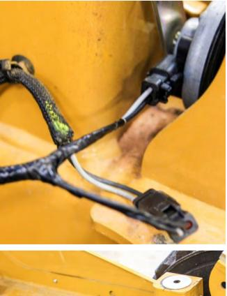
E. Feed the wiring along the existing horn harness and secure them to each other with zip ties.
