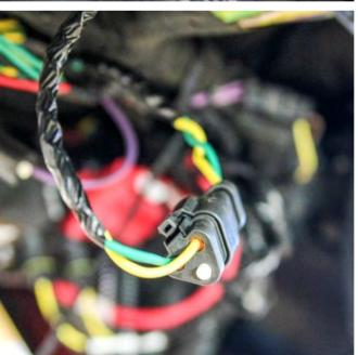
Locate the existing CAT Delphi PA66 connector behind the Machine Interface Module, on the left side.
