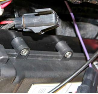
K. Remove the connector cover to expose the 15 amp fuse.
