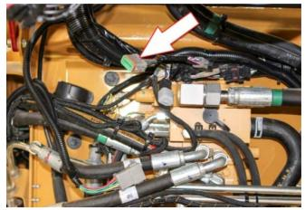
B. Plug the male connector C201into the female connector C102.
