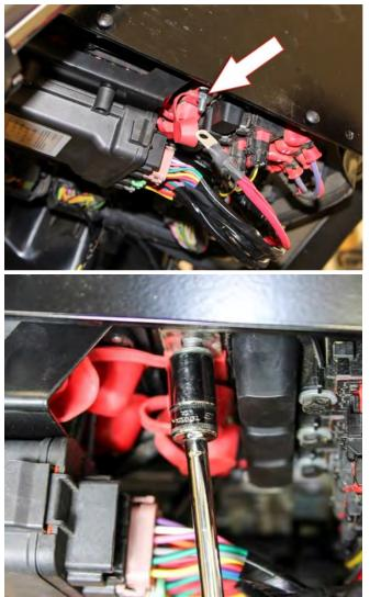
C. Use the 13mm socket to remove the existing nut and washer from the bolt.
