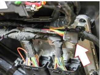
D. Remove existing CAT Deutsch connector from cover or CAT Product Link module.
