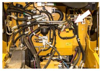
B. Use needle nose pliers to pull the red tab up to unlock the rectangular connector.
