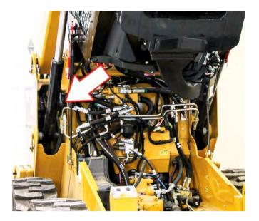
C. Feed connector C202 through the right side of the machine, along the existing electrical lighting harness running to the rear right tail light.
