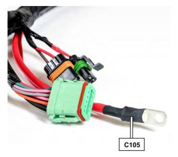
B. Locate the right bolt below the Machine Interface Module and remove the boot.
