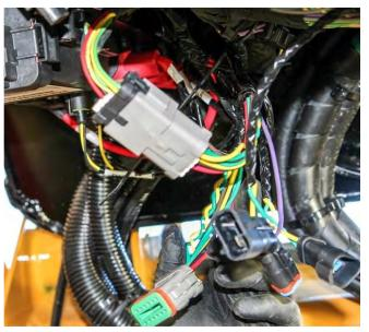
F. Attach Machine Interface Harness Deutsch connector C509 to the existing Deutsch connector cover (or Product Link Module if equipped).
