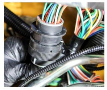
C. Plug the MIH rectangular connector into the rectangular female connector that was previously mated to the bulkhead connector. Engage the red retainer.
