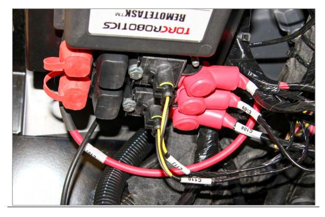
7. Verify that the connectors and bolts in steps 4-6 are secured.
