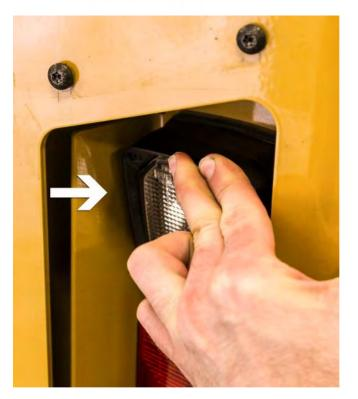
C. Feed the UIH Deutsch connector through the opening to the left of the rear lights. Pull the harness through to allow enough length to reach the REI.
