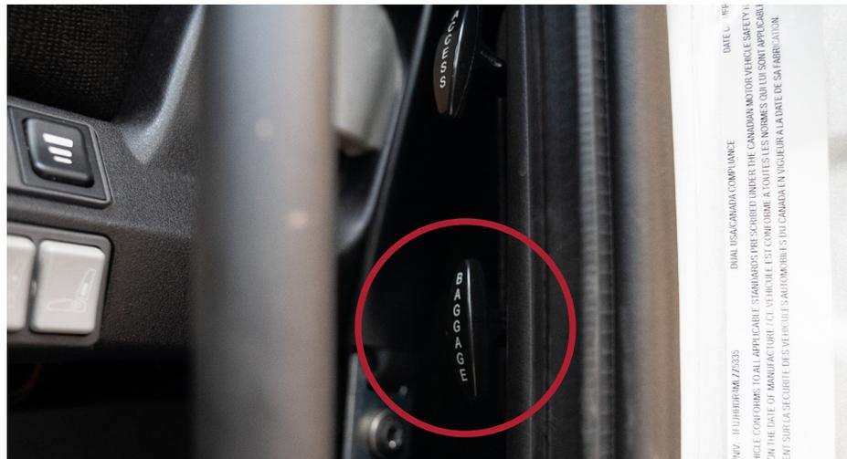
Figure 16. Driver-side baggage compartment pull cable
