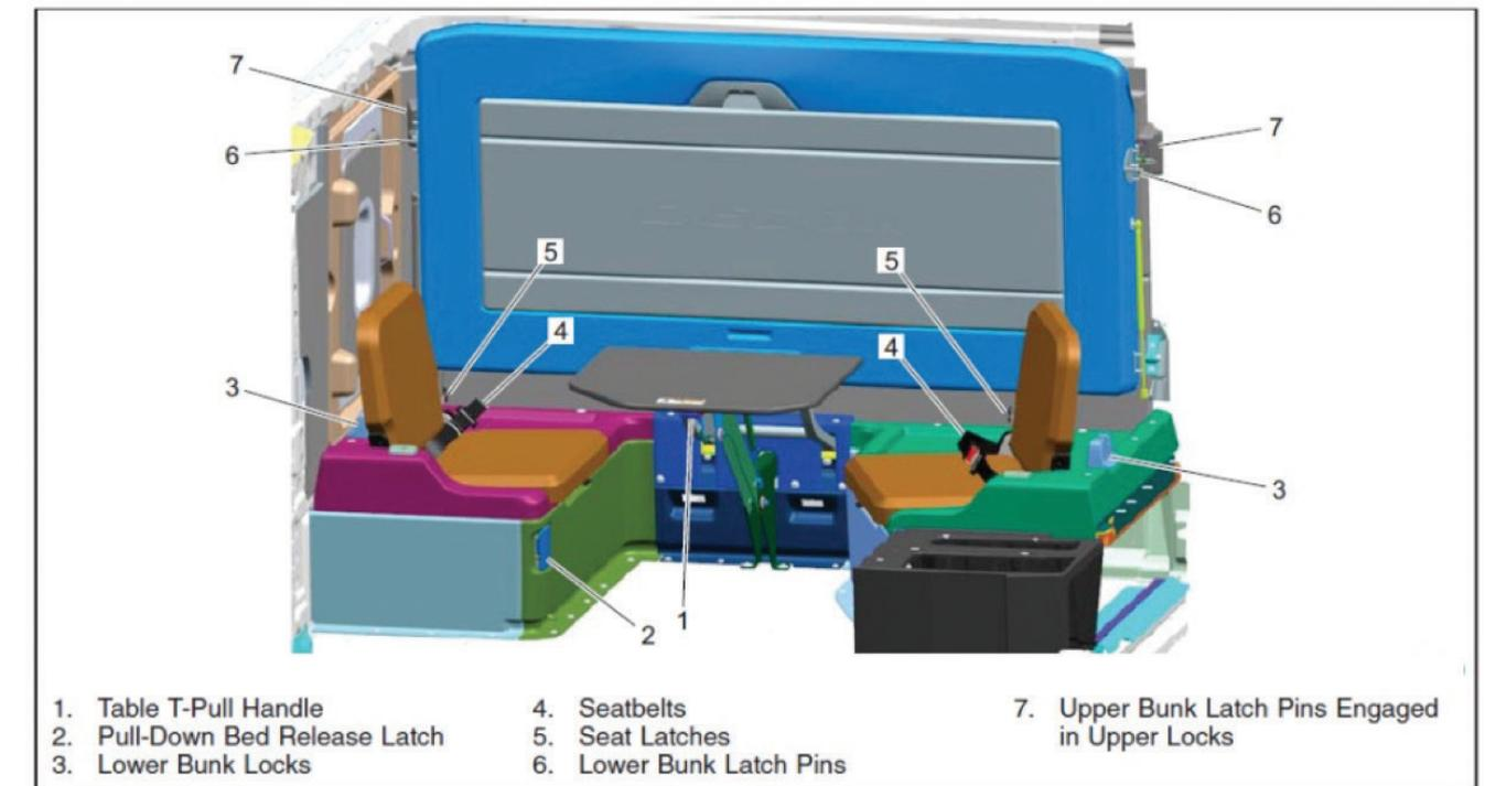
Figure 7. Rear passenger seats (DTNA, 2023)
