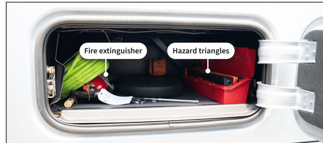
Figure 14. Location of hazard triangles and fire extinguisher
