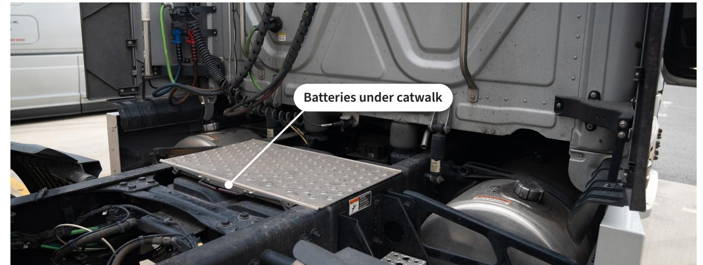
Figure 23. Location of batteries under catwalk
