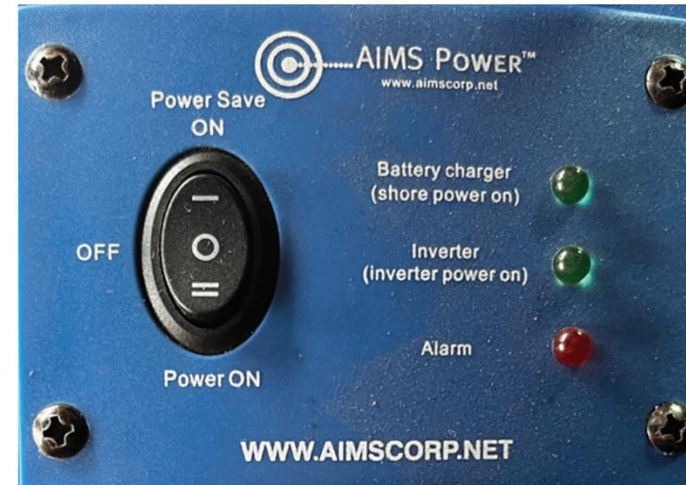
Figure 18. AC power switch (O is OFF)
