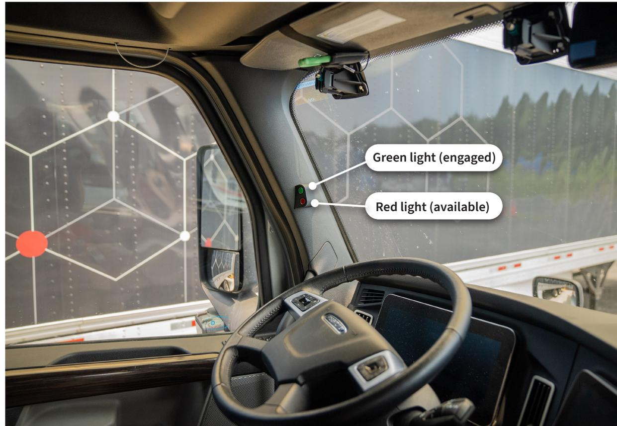
Figure 3. ADS indicator lights – A-pillar
