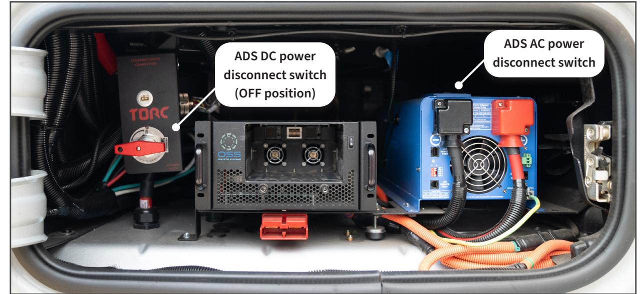
Figure 17. Location of DC and AC power disconnect switches
