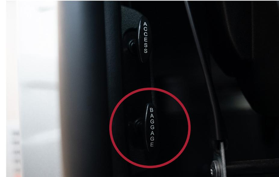
Figure 13. Passenger-side baggage compartment pull cable
