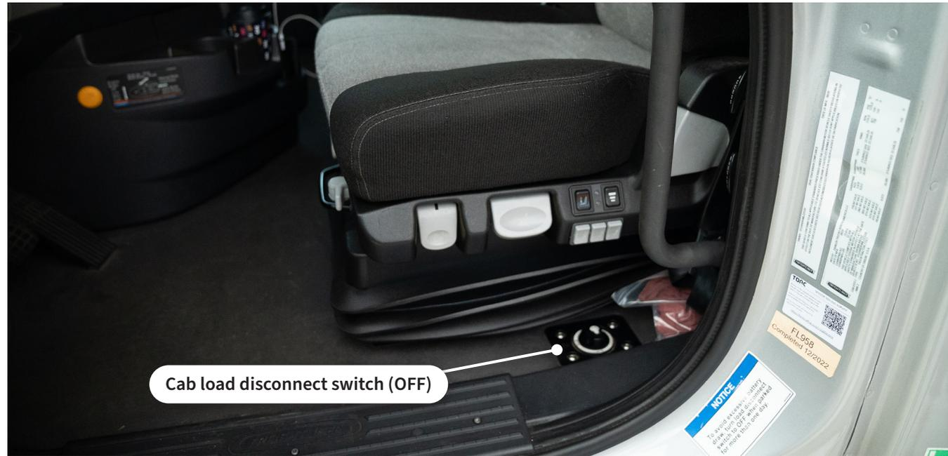
Figure 21. Location of the cab load disconnect switch
