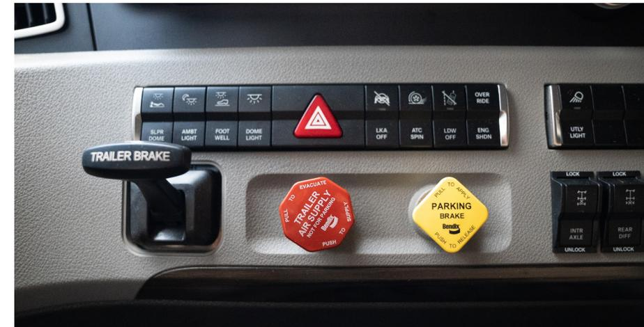
Figure 9. Brake valve control knobs
