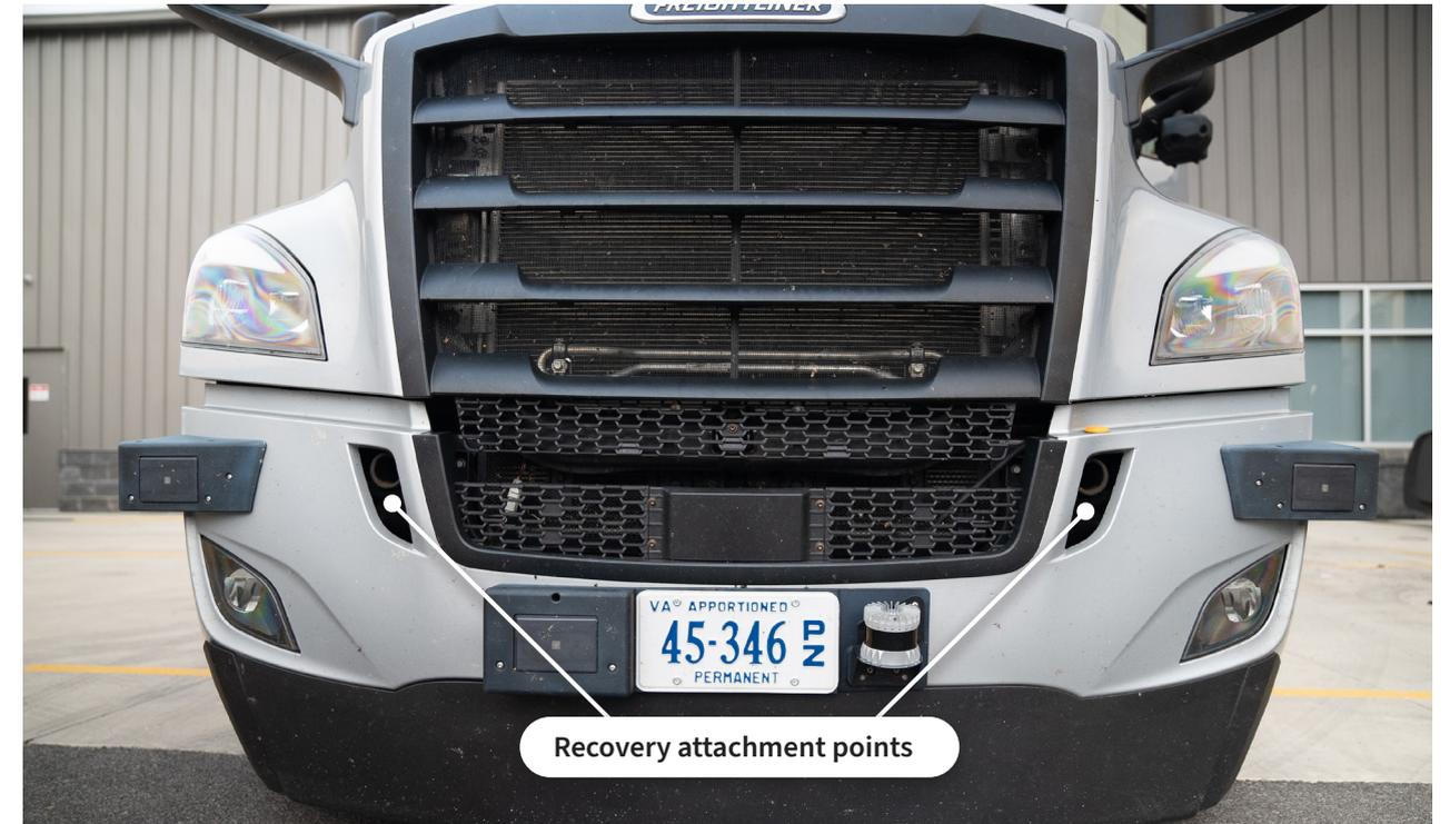
Figure 20. Freightliner Cascadia recovery attachment points
