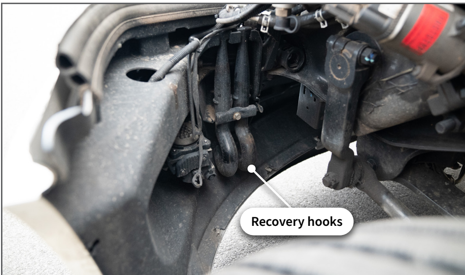
Figure 20. Recovery hook location
