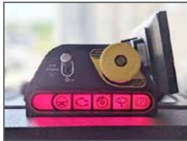
Figure 11. Emergency Manual Override (EMO)
