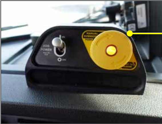
Figure 4. Emergency Manual Override (EMO)
