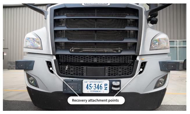
Figure 20. Freightliner Cascadia recovery attachment points
