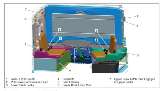
Figure 7. Rear passenger seats (DTNA, 2023)
