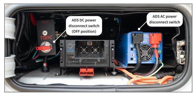
Figure 17. Location of DC and AC power disconnect switches
