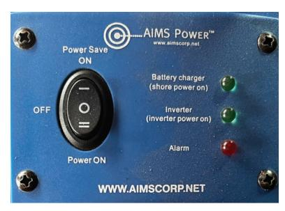
Figure 18. AC power switch (O is OFF)
