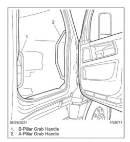
Figure 6. Passenger-side entry (DTNA, 2023)
