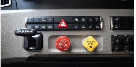
Figure 9. Brake valve control knobs
