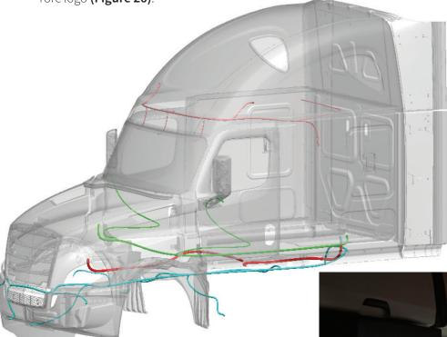
Figure 25. Electrical wiring diagram
