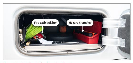
Figure 14. Location of hazard triangles and fire extinguisher
