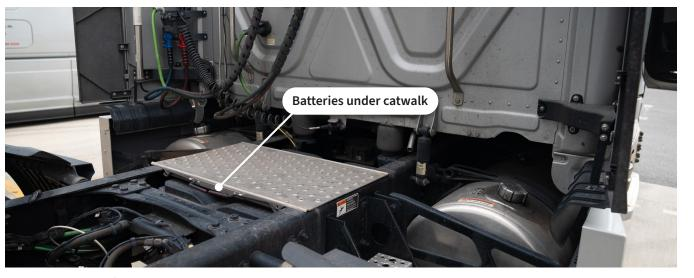
Figure 23. Location of batteries under catwalk
