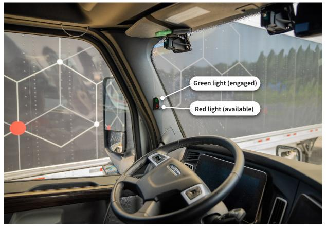
Figure 3. ADS indicator lights - A-pillar
