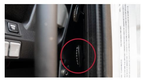
Figure 16. Driver-side baggage compartment pull cable
