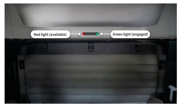
Figure 4. ADS indicator lights – rear overhead
