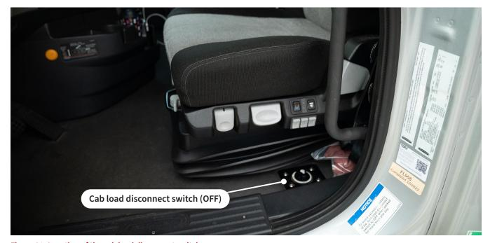
Figure 21. Location of the cab load disconnect switch
