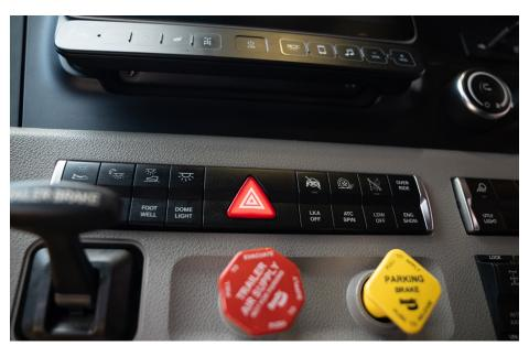
Figure 11. Hazard Warning Signal Flasher
